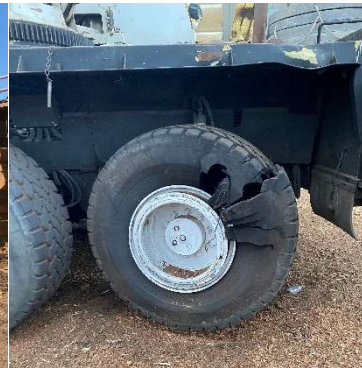
The ruptured rear tire that injured the employee.
