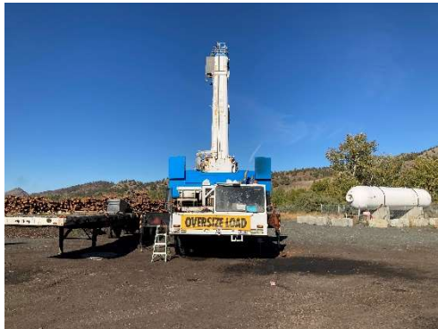
The Demag AC 335 165-ton mobile crane.
