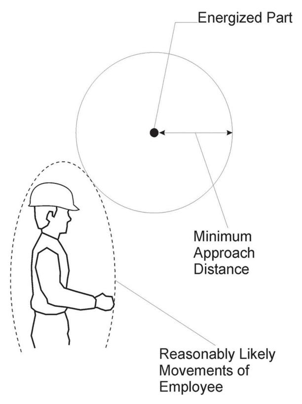
Figure 1 - Maintaining the Minimum Approach Distance
