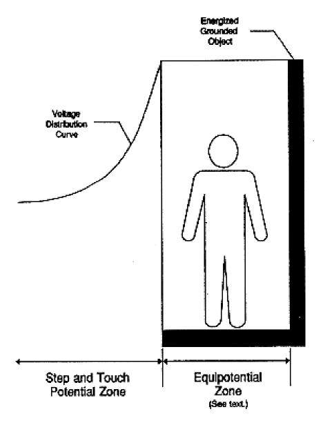
Figure 3 - Protection from Ground-Potential Gradients
