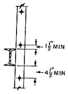
Figure 4. Clearance for Unavoidable Obstruction at Rear of Fixed Ladder
