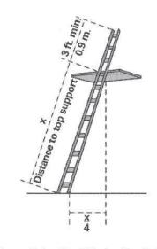
Figure D-1 -- Portable Ladder Set-up
