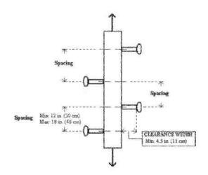
Figure D-6 - Step Bolt Spacing
