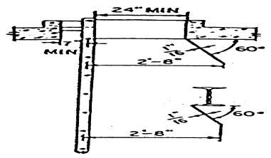
Figure 6. Deflector Plates for Head Hazards
