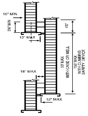
Figure 11. Offset Fixed Ladder Sections
