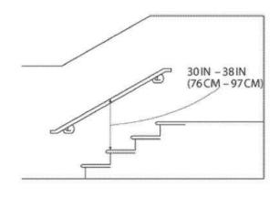
Figure D-12 - Handrail Measurement
