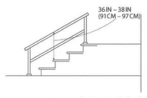
Figure D-13 - Combination Handrail and Stair Rail
