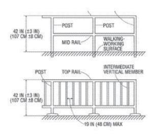
Figure D-11 - Guard Rail Systems
