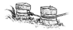
Figure 7-21 - Stump Tie Back Anchor
