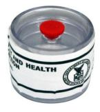
Sealed cassette allows access to inlet/outlet ports after sample has been taken.
