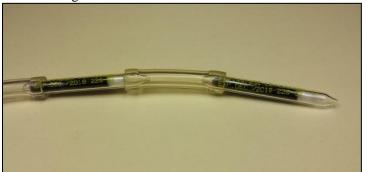
Figure 3. Two Charcoal Tubes in Series
