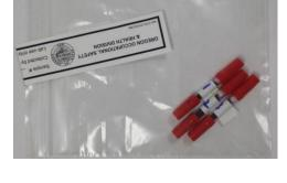
Charcoal tubes inside of a Whirl-Pak® with bag opening securely closed and sealed. Other media types, such as filter cassettes and bulk solid material (e.g. paint chips), may be sealed in this manner. Charcoal tubes in zip lock bag allow access to samples because bag opening not completely sealed.
