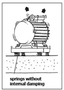
Figure 34. Isolated Structure-Borne Noise
