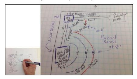
Figure 26. Drawing a Noise Diagram
