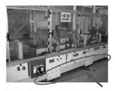
Seal off all small gaps and openings along all polycarbonate panel edges and the adjacent framework, and the bottom edge of the machine cabinet to the floor.
