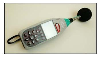
Most Type 1 and Type 2 sound level meters can be set to respond with either a "slow response" or a "fast response." The meter dynamics are such that the meter will reach 63% of the final steady-state reading within one time constant:
