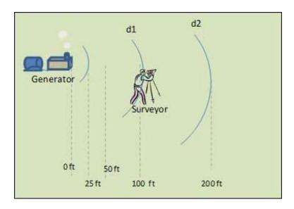
*Example:* A worker is surveying an open field, which has a diesel generator running in the middle of it. The worker is 100 ft from the generator and is exposed to a noise level of 85 dBA. When the worker is 25 ft from the generator, the noise level will be 97 dBA. At 200 ft from the generator the worker will be exposed to a noise level of 79 dBA.
