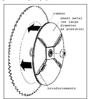
Figure 33. Adding Damping Material to a Saw Blade
