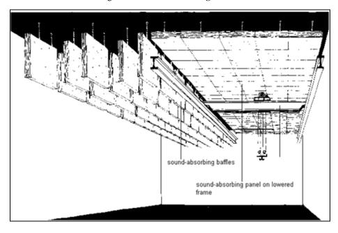
Figure 38. Sound-Absorbing Baffles
