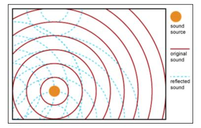
Figure 5. Original and Reflected Sound Waves
