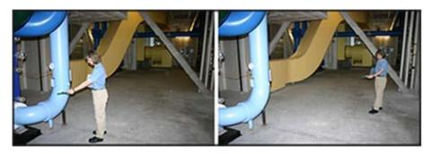
Your completed sketch will show a series of contours around the noise source(s) (Figure 26). Expect the contours for adjacent noise sources to overlap. Workers operating entirely outside the contour are not exposed to noise in excess of the AL. Workers whose tasks take them closer to the equipment might experience exposures between the AL and the PEL, or even in excess of the PEL. Take photographs to document the type of equipment or process.
