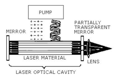
Figure III: 6-1. Components of a Laser
