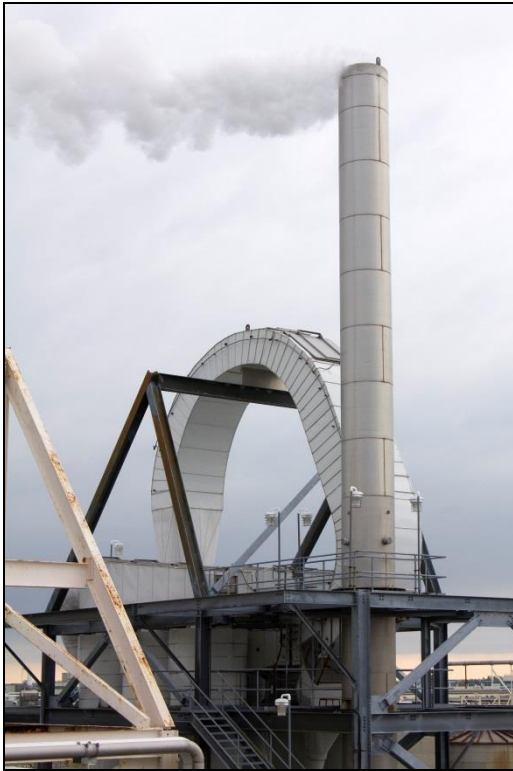
Figure II.18 A Ring Dryer
