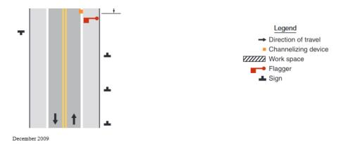
Figure 6C-3. Example of a One-Lane, Two-Way Traffic Taper
