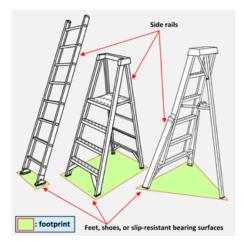
support. They have larger footprints than non-self-supporting ladders because they have front and rear side rails. Design styles such as stepladders, platform ladders, and double front ladders have footprints that can be placed adjacent to vertical surfaces such as walls. This can be an advantage over non-self-supporting ladders such as extension ladders that require the footprint to be set back from the upper-support surface to achieve a safe ladder angle.
