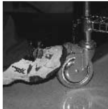
▲ Jammed wheel, faulty brake
