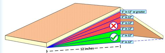
The type of fall protection that employees must use on low-slope roofs depends on the distance they work from the roof edge. (An unprotected skylight is also considered a roof edge.) There are three zones:
