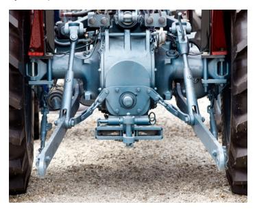
Before servicing, adjusting, cleaning, or unclogging the equipment, stop the engine, disconnect the power source, and wait for the PTO shaft to stop, except when the machine must be running properly to be serviced or maintained. In that case, the employer must train workers on all steps and procedures needed to safely service or maintain the equipment.
