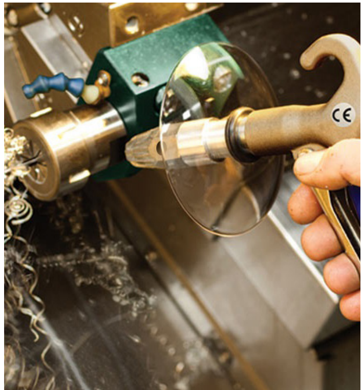
Nozzle designed with a built-in protective air cone. (Image: Guardair Corporation)
