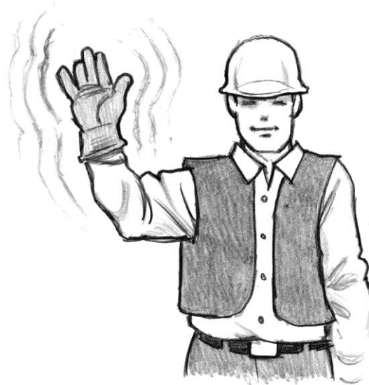
Figure 7-54 – Mainline Ahead (One arm raised, hand fluttering)
