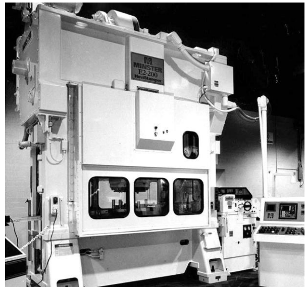
Straight side press with automatic feeding equipment and guards that totally enclose the die area (with Lexan panels). Source: Minster
