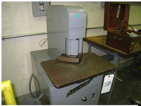
Notching machine with guard.
