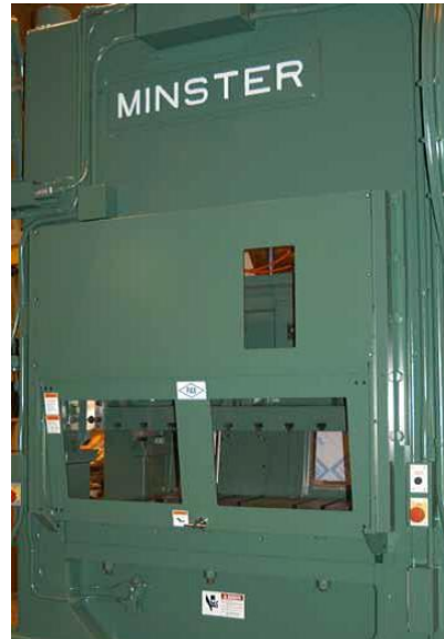
Interlocked barrier guard on a straight side press. Source: Minster
