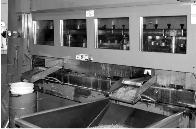
Interlocked barrier guard on a large straight side press. Note the adjustable bottom panel that allows for differing part and scrap discharge points. Source: Minster
