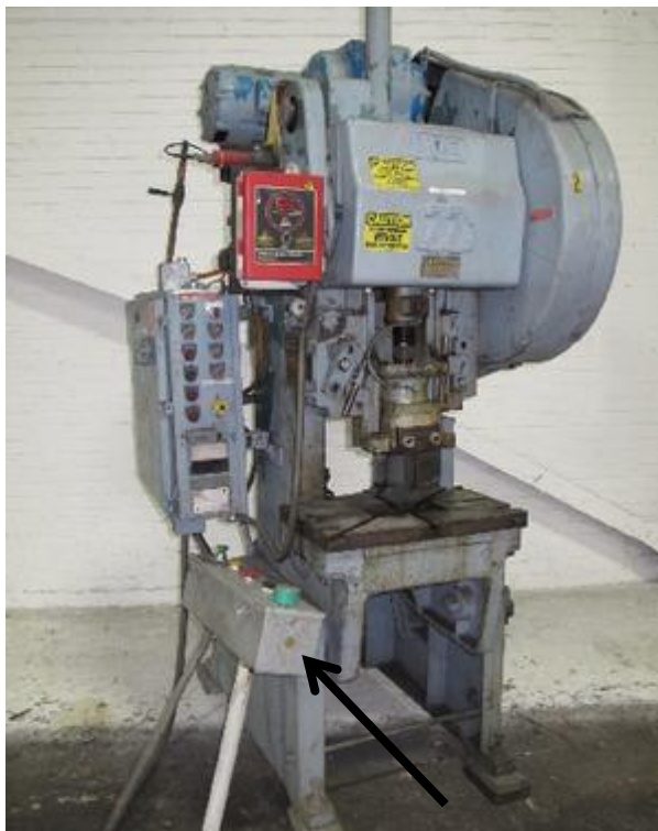
Two hand trips can be effective safeguarding but may not be ergonomically correct. Notice the twisting that would occur on this mechanical power press. 1910.217
