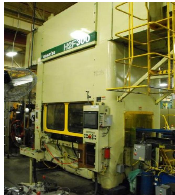
This is a direct drive, servo-motor, straight side power press. Direct drive presses don't have flywheels, belts, or clutches but rather a high torque, low rpm servo motor powering a driveshaft, main gear, and crankshaft. OSHA considers them a part revolution mechanical power press. 1910.217
