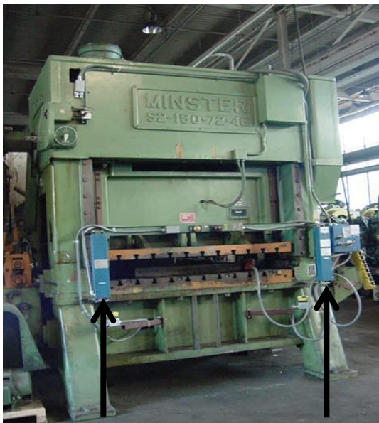
A presence-sensing device, or light curtain, on a straight side mechanical power press.
