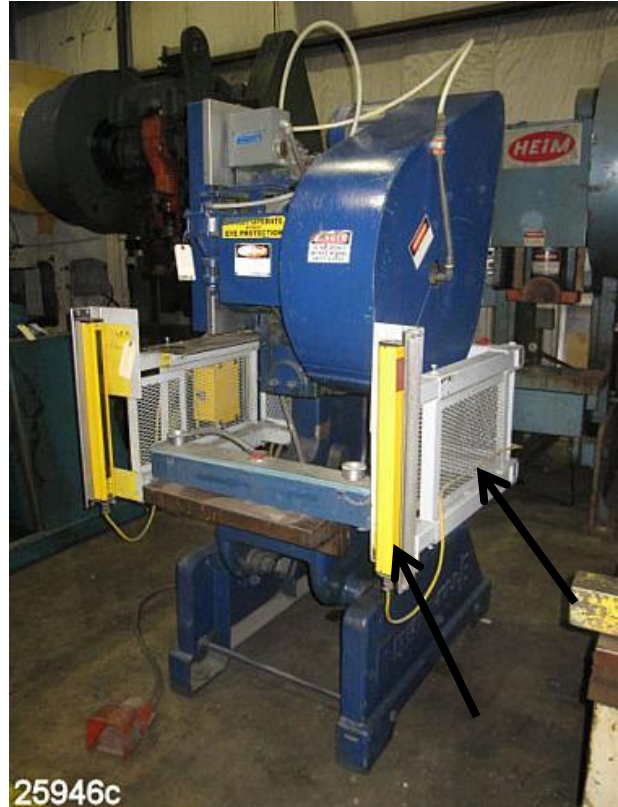
Light curtains and fixed barrier guarding on a gap frame mechanical power press (OBI). 1910.217
