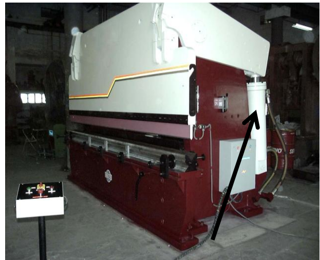
Hydraulic press brake. Note the arrows pointing to the hydraulics. 1910.212 and P.D. A-217
