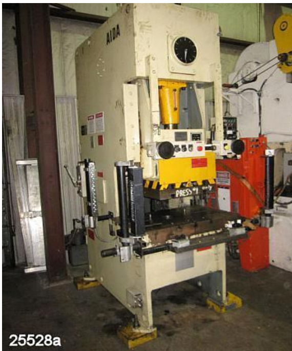
Although this looks like it could be a hydraulic press, it's actually a gap frame – open back stationary (OBS) mechanical power press (mechanical components are inside frame). Light curtains indicate a part revolution clutch. 1910.217
