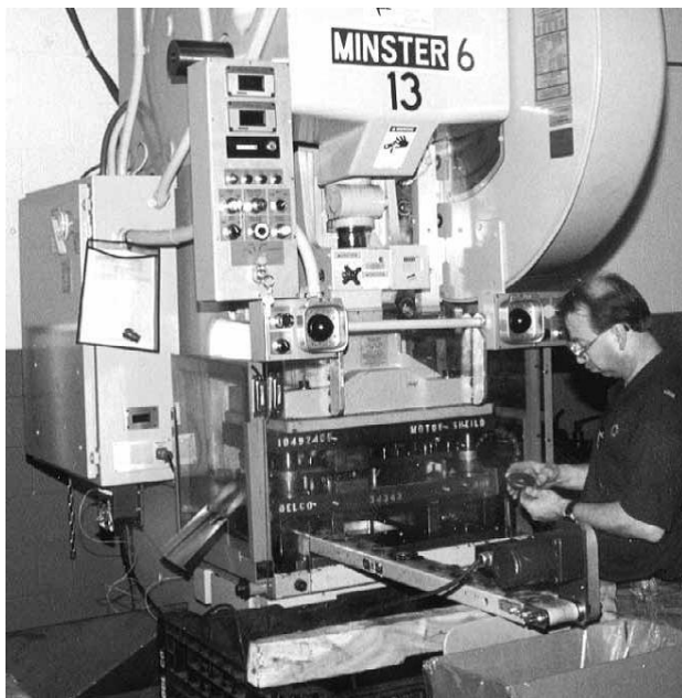
A gap frame press in automatic production mode using an interlocked Lexan barrier guard. Source: Minster
