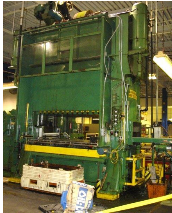
Back view of a straight side mechanical power press. 1910.217
