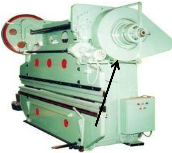
Mechanical press brake. Note the arrow pointing to the flywheel. 1910.212 and P.D. A-217
