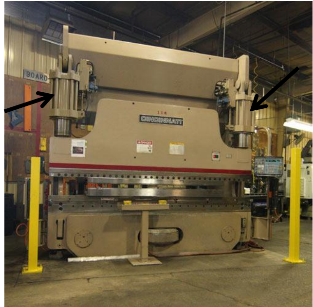
Hydraulic press brake. Note the arrows pointing to the hydraulic cylinders. 1910.212 and P.D. A-217
