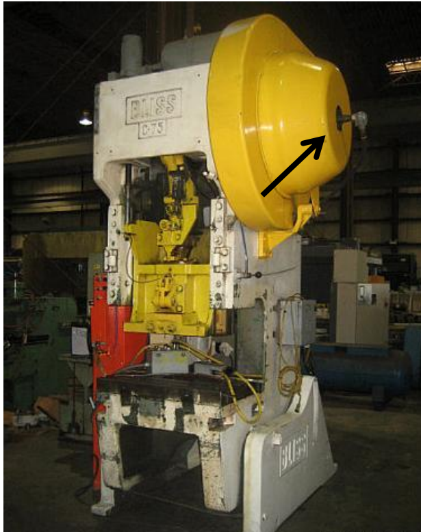
Airline to flywheel/clutch indicates a part revolution mechanical power press. 1910.217
