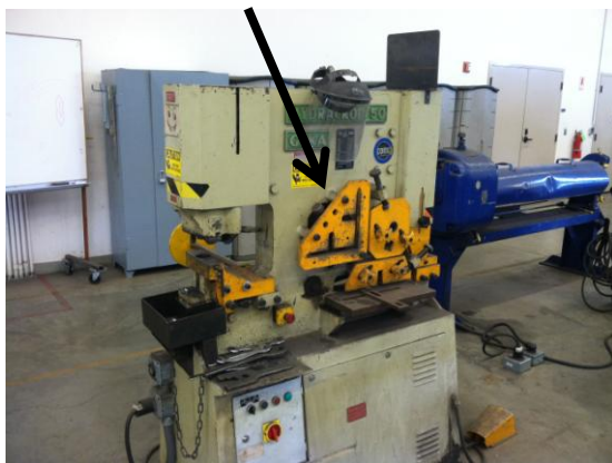
Ironworker with adjustable guarding. Source: Lane Community College
