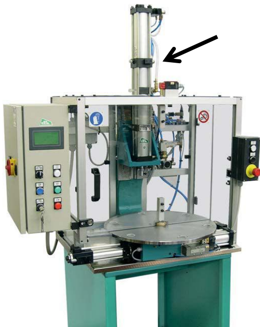
Pneumatic press. The arrow shows the air ram. 1910.212
