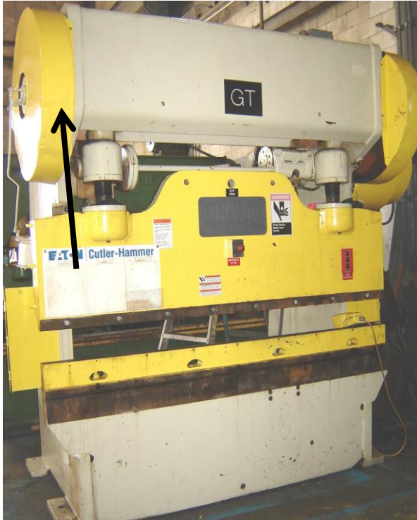
Mechanical press brake. Note the arrow pointing to the flywheel. 1910.212 and P.D. A-217
