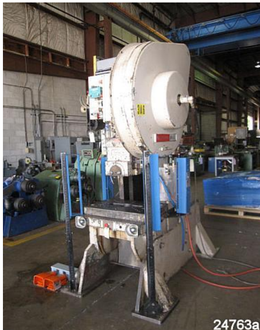
This part revolution press depicts the airline going into the flywheel/clutch assembly – an easy way to tell it's a part revolution press.
