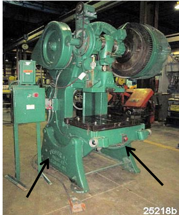
Gap frame mechanical power press. Open back incline (OBI). 1910.217. Arrows depict where the press can swivel back.
