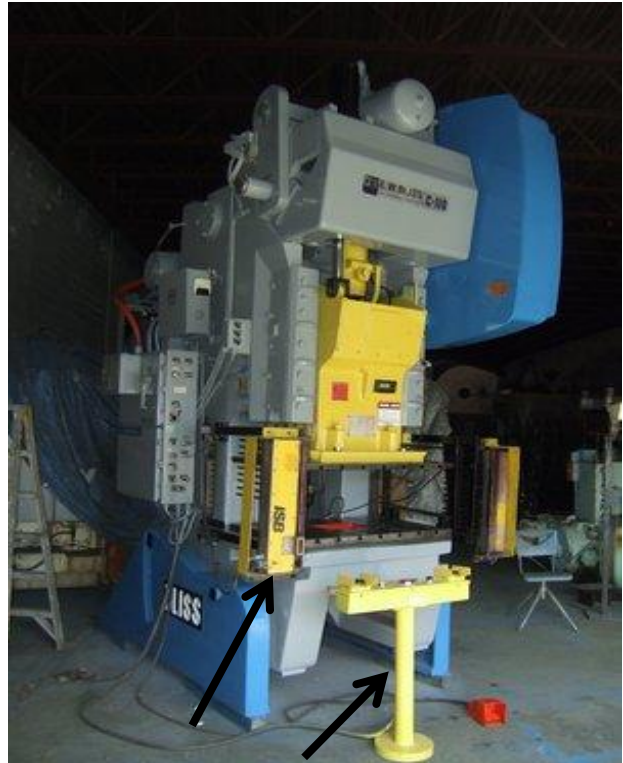
Control stand in addition to light curtains on a part revolution mechanical power press. 1910.217
