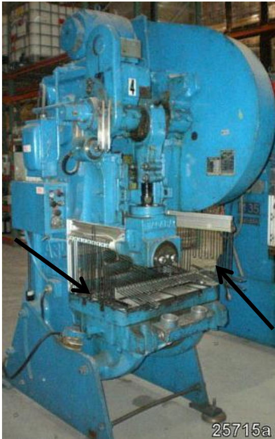
Adjustable guarding on a gap frame mechanical power press. Open back incline (OBI). 1910.217
