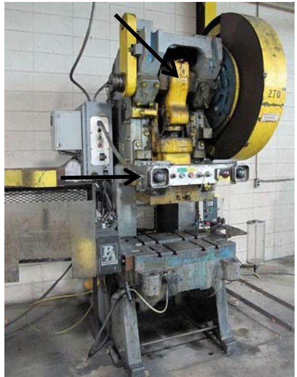
A good look at the flywheel, crankshaft, and two hand controls/trips on this mechanical power press. 1910.217
