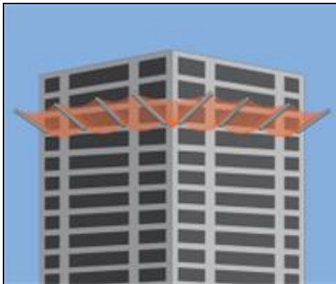
Figure 12. Safety net system
