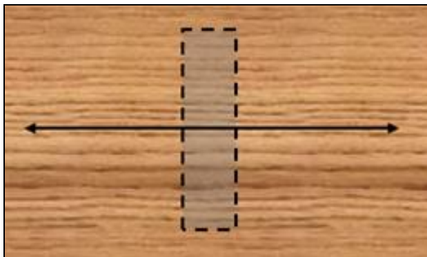
Figure 10. Plywood orientation relative to hole orientation and strength axis
