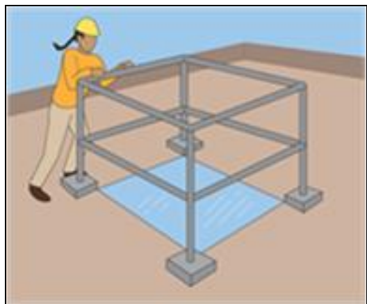
Figure 2. Guardrail used around an opening
