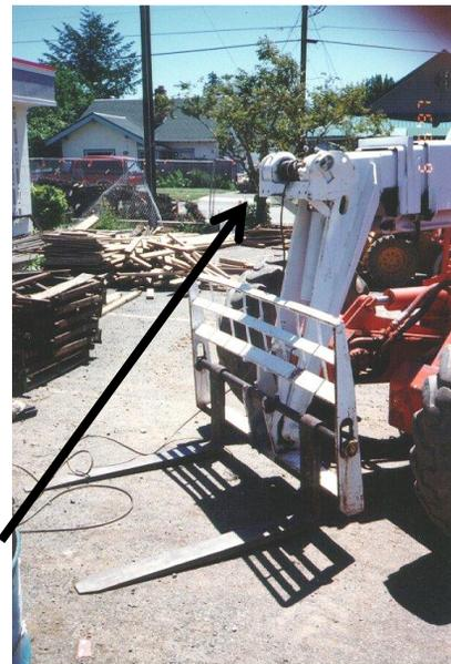
*A winch was welded on the boom of this telescoping truck without the manufacturer's approval.*
