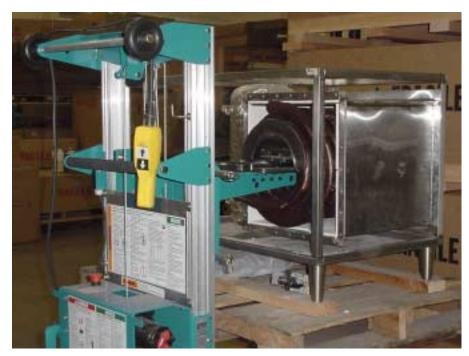
The end device of the coil lifter is pushed forward and easily glides the coil (weighing 110 lb.) into the heat exchanger shell. This eliminates all manual lifting and handling of the coil while inserting it.
