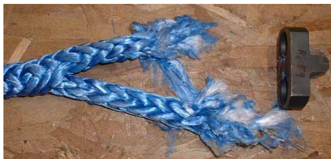
Figure 53. Failed knuckle link after break test
