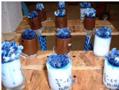
Figure A3. First potting attempt with Phillystran Socketfast ® Blue A-20
