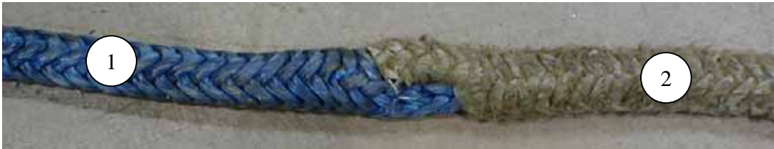
Figure 9. Finished long splice
