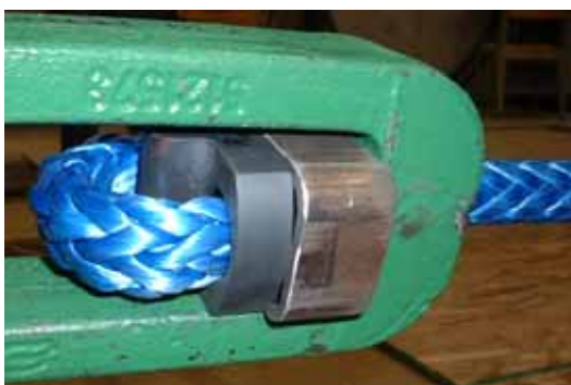
Figure 52. Knuckle link in test block with test collar before break test
