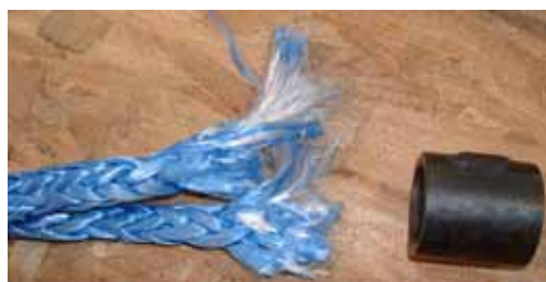
Figure 51. B) Pinned nubbin after break test
