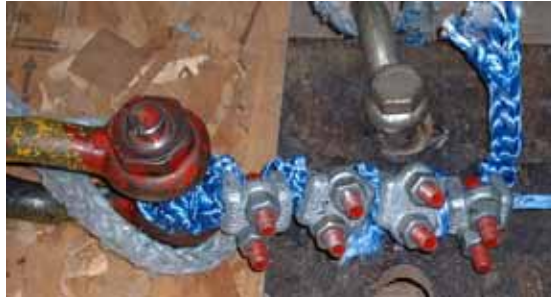
Figure 54. Test specimen exhibiting rope clamp slippage after a break test
