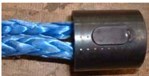
Figure 51. A) Pinned nubbin before break test
