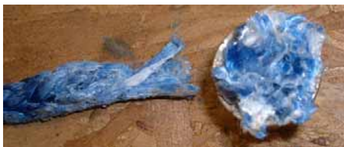
Figure 56. Failed notched nubbin sample where 10 of 12 strands failed
