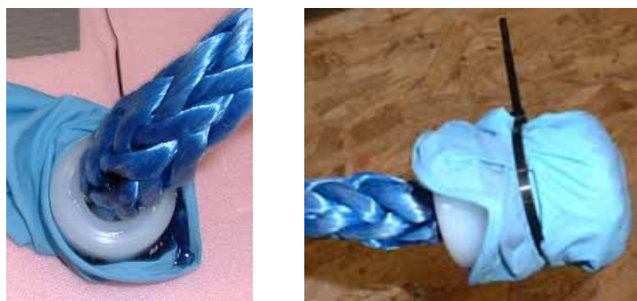
Figure A4. A) UHMW-PE nubbin with Phillystran adhesive potting in mold B) Potted UHMW-PE nubbin with Phillystran adhesive
