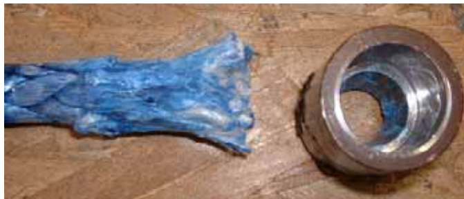
Figure 55. Failed notched nubbin sample where bond did not hold
