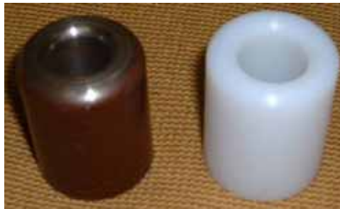
Figure 15. B-5 Steel nubbin and UHMW-PE nubbin
