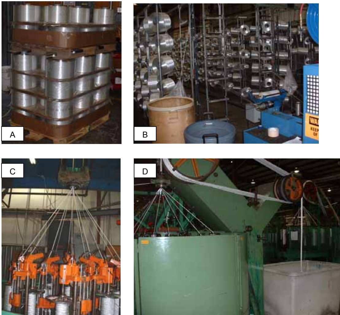
Figure 1. A) Fiber delivered in spools B) Fiber spun into yarns C) Yarns spun into strands D) 12 strands braided into (uncoated) finished product
