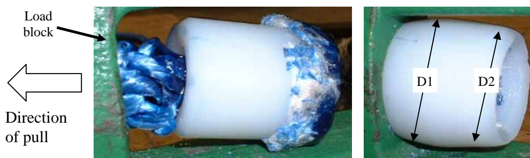
Figure 57. UHMW-PE nubbin before and after load test
