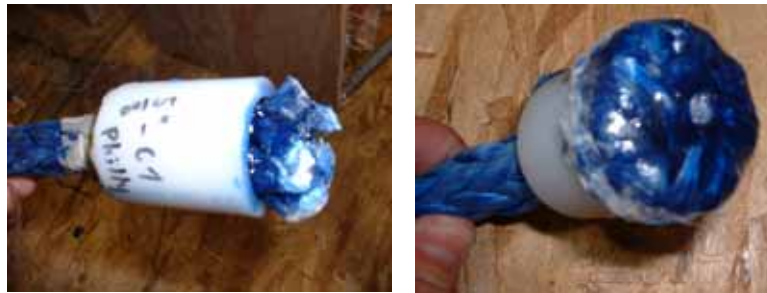
Figure A5. A) First potting attempt with Phillystran adhesive B) Potting technique used in pilot study
