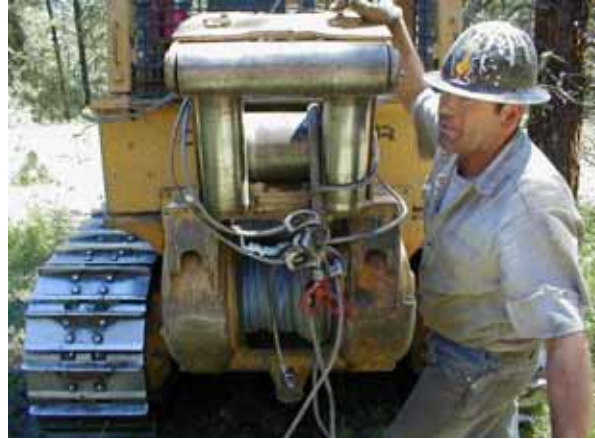
Figure 8. Synthetic rope winchline with slider style chokers
