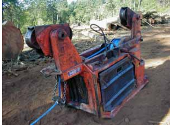
Figure 10. Synthetic rope on Boman Mark IV internal drum carriage
