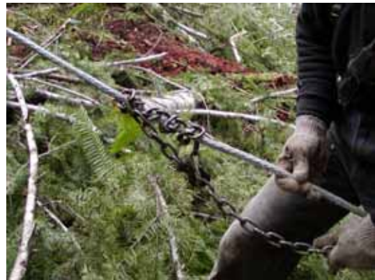
Figure 4. Use of a rigging chain for tightening a synthetic guyline
