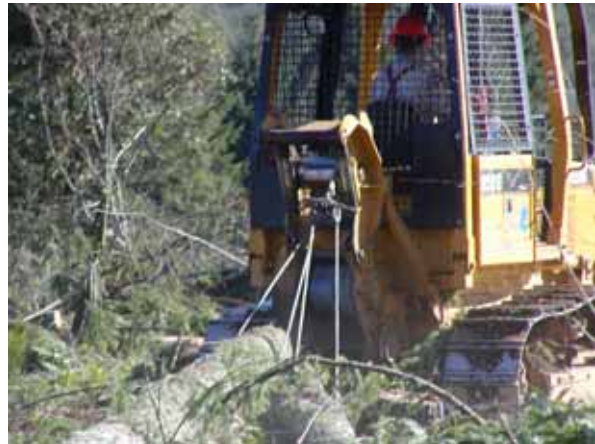
Figure 9. Synthetic rope winchline with ring style chokers
