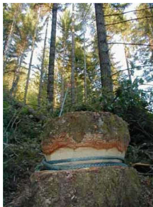
Figure 5. Synthetic intermediate support line
