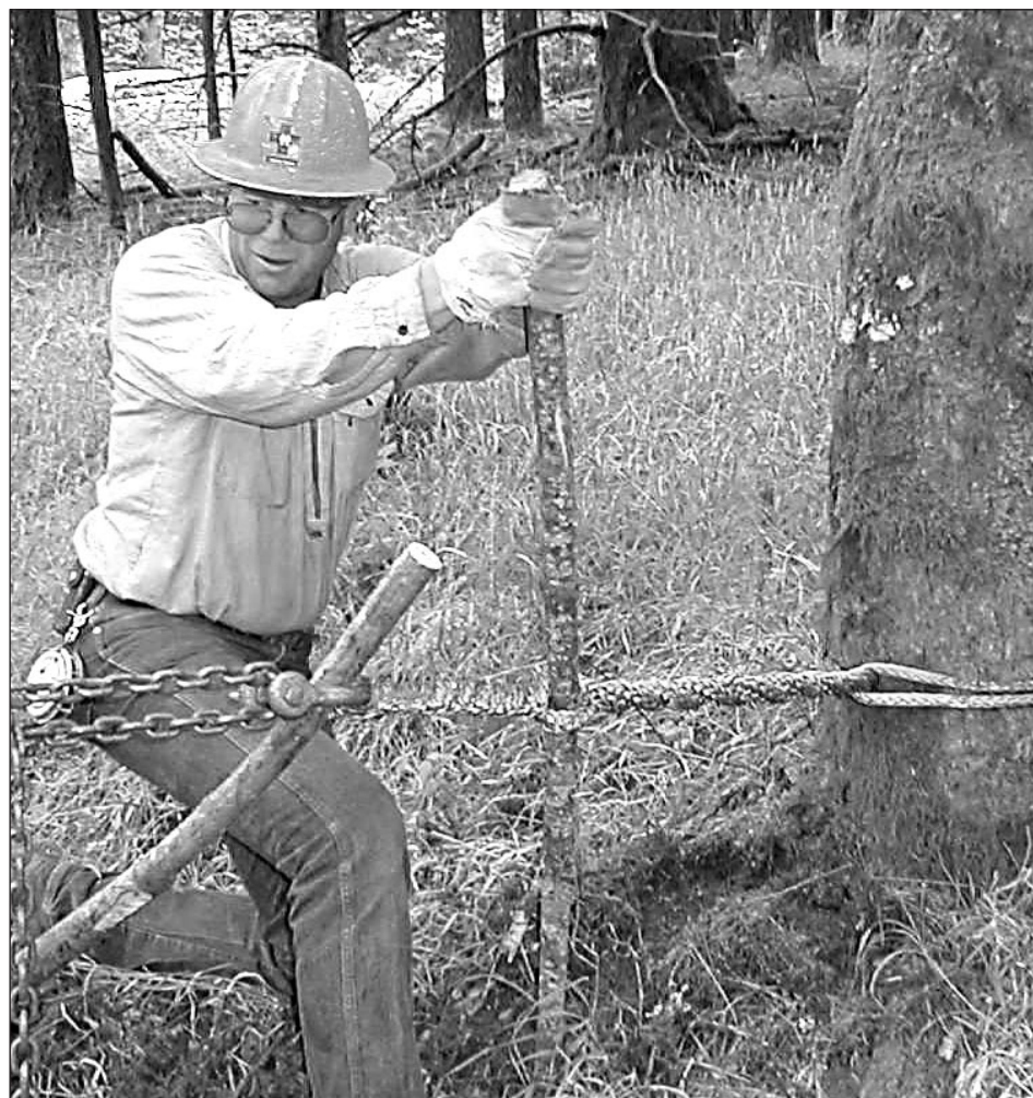
STEVE PILKERTON, researcher at OSU, setting a "twister" with synthetic rope. OSU researchers are in the second installment of research on the synthetic line's potential uses and how it functions in real world logging conditions. To date, the results appear to be promising, with more research to be completed over the next two years.
