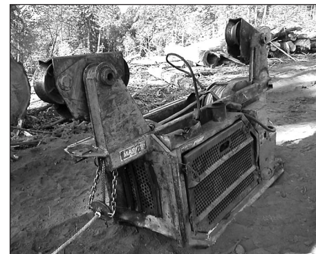
AMSTEEL in use as dropline on this motorized carriage.
