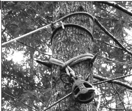
INTERMEDIATE supports and supporting guylines using synthetic line... easier rigging.
