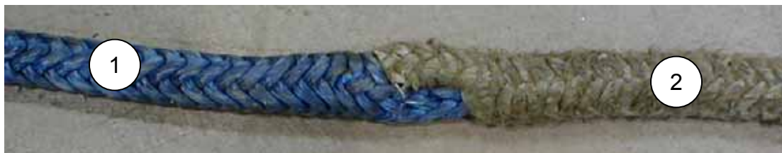
Figure 5. Finished long splice
