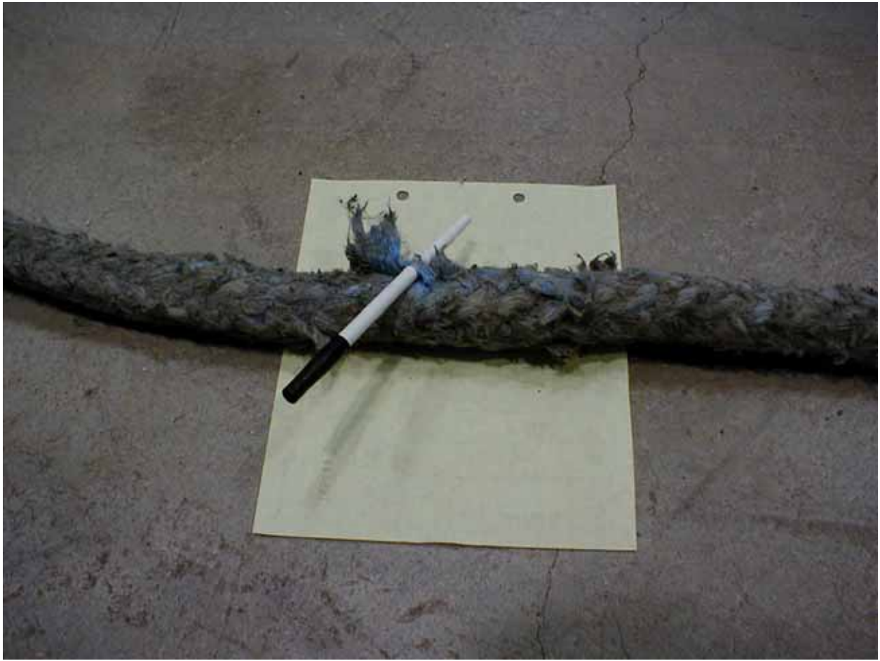
Figure R9. Severe abrasion in a section of 7/8-inch ASB synthetic winch line. Pen is inserted underneath the intact remnants of a strand. Manufacturer's recommendation is to retire a rope or cut and re-splice the remaining rope when 2 or more adjacent strands are cut.
