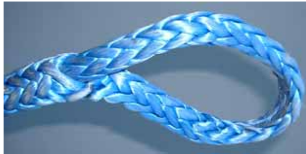
Figure 1. Buried eye splice
