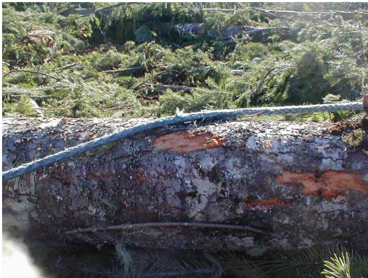
Figure R14. Rubbing on log shows sources of abrasion in operation and need for planning of extraction to prevent abrasive locations and to plan the lead to avoid rubbing on standing timber or over stumps.
