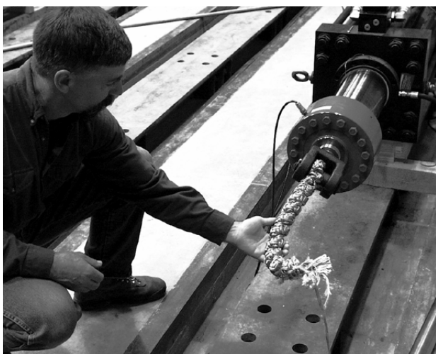
Figure 2. Failed test section showing break at the end of splice.
