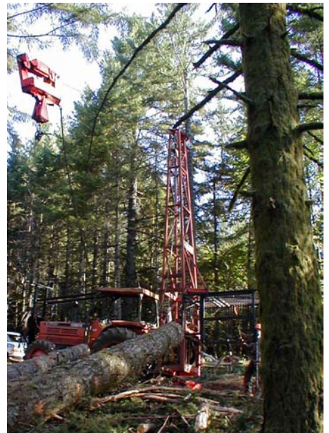
Figure 2. Koller K300 yarder, SKA-1 carriage, and yarded turn at landing.
