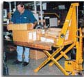
▲ Scissors lift provides a portable, height-adjustable workstation
