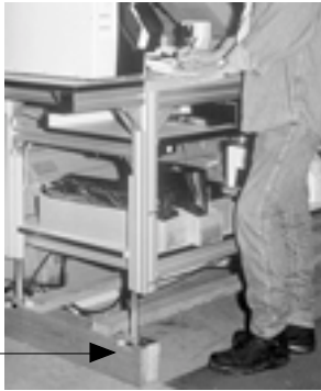
Raise the work surface
