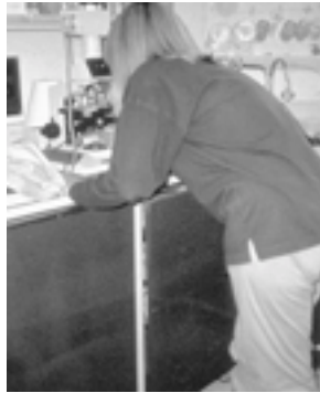
Microscope workstation — leads to uncomfortable work posture with bending
