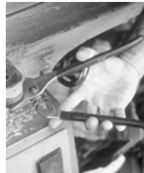
Using a hand tool — grip span too wide
