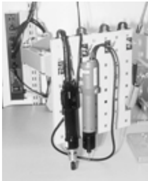
Triggerless tools — contact switches replace triggers
