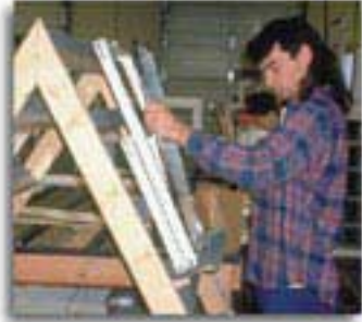
▲ Simple wooden A-frame makes work more comfortable and efficient
