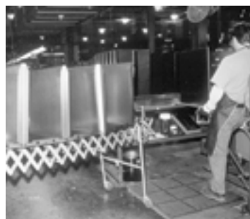
Portable roller conveyor — eliminates carrying of products between workstations
