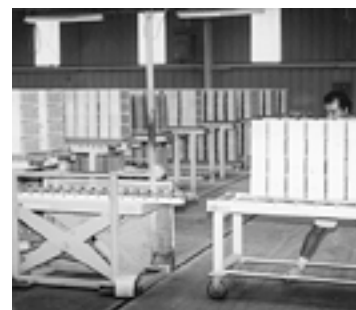
Roller conveyors on a cart and scissers lift — replaces lifting and carrying with rolling and sliding
