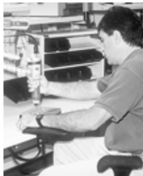
In-line tool — can be used with a straight wrist on horizontal surfaces
