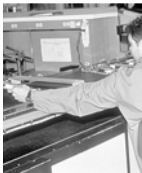
Work too far away — extended reach
