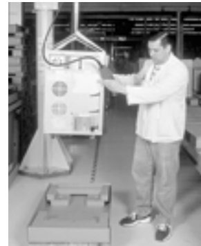
Workstation crane for heavy loads
