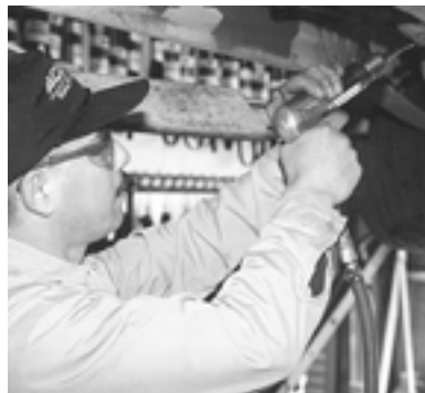
Hand-arm vibration — pneumatic chisel
