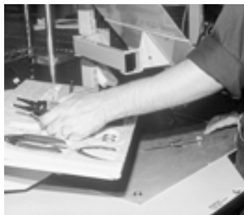
Foam tool pad on adjustable tray — employees cut out the foam and arrange their own tools. Reduces reaching for frequently used tools and eases pressure points on the hands and fingers
