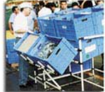
▲ Parts storage is tilted for easy access and convenience
