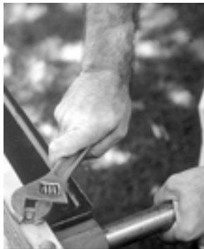
Using a hand tool — bent wrist
