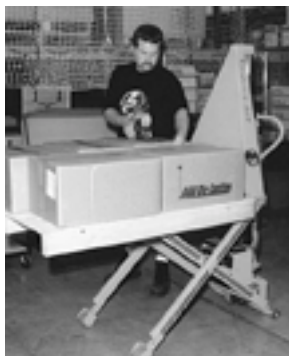
Maintaining comfortable, midrange working postures
