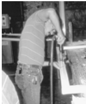
Using a pistol grip tool on a horizontal surface — awkward upper body posture and bent wrists
