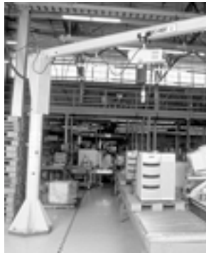
Workstation crane for heavy loads
