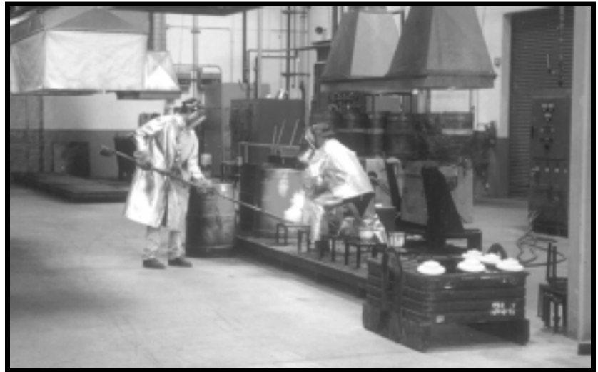
A part of the casting process is the foundry pour where molten metal is poured into molds.
