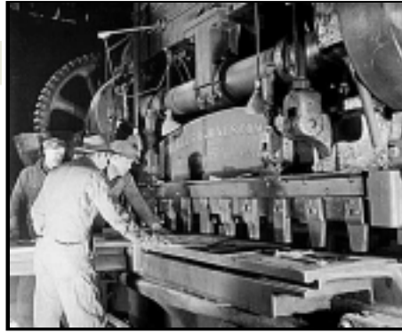
1941 – Workers at an Eastern shipyard operate a giant shear to shape steel parts for the US Liberty Fleet in 1941.
