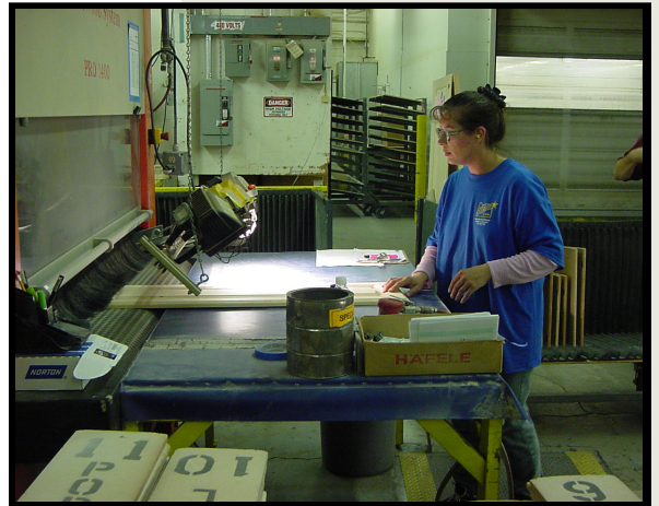
Employees of Masterbrand in Hillsboro work together to craft kitchen cabinets one step at a time. Here, a worker is fine-sanding a cabinet door.
