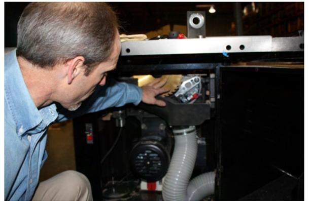
Steve Gass shows how a mounted cartridge works inside the table saw.
