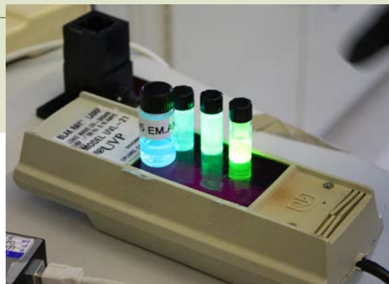
Qdot® Nanocrystals are one of several chemical technologies developed at the company. The size of the dot determines the color when placed under a black light.
