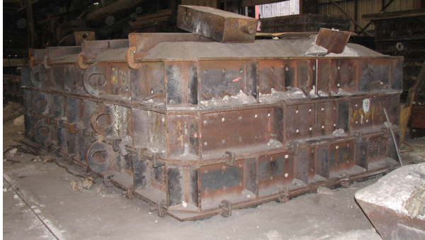
The mold minus two of the 18-inch layers that were in use when the accident occurred.
