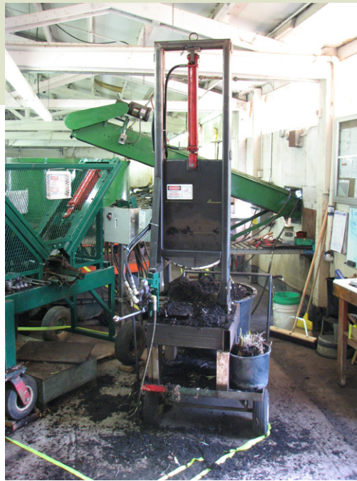
This root divider was not properly guarded.
