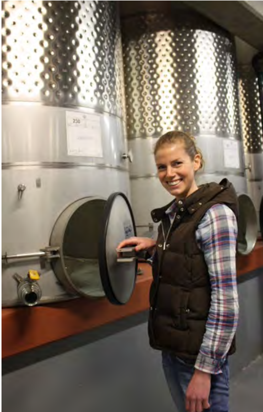
Above: Tracy Faulds said workers never have to enter tanks at Adelsheim because of the access door at the bottom.
