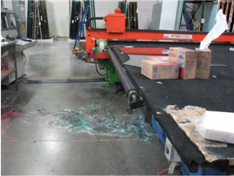
The lower section of the plate glass shattered on the ground. The upper section fell on the table.
