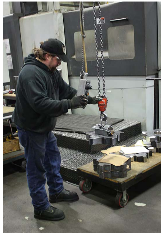
Above: Custom guards were made to keep workers from reaching inside this piece of machinery. Center: Ryan Morgan uses an overhead crane to lift a 60-pound blade segment. Right: Michael Flinker pulls parts to build an assembly. Top Right: Cecil Smith performs his work on a table that has been lifted so he doesn't have to bend over repeatedly.
