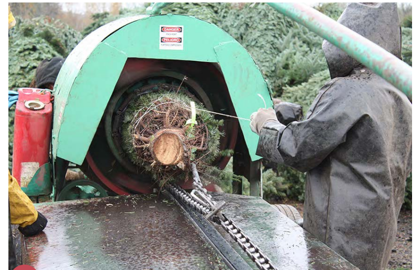
3 Christmas trees make their way through a baling machine before being shipped out.
