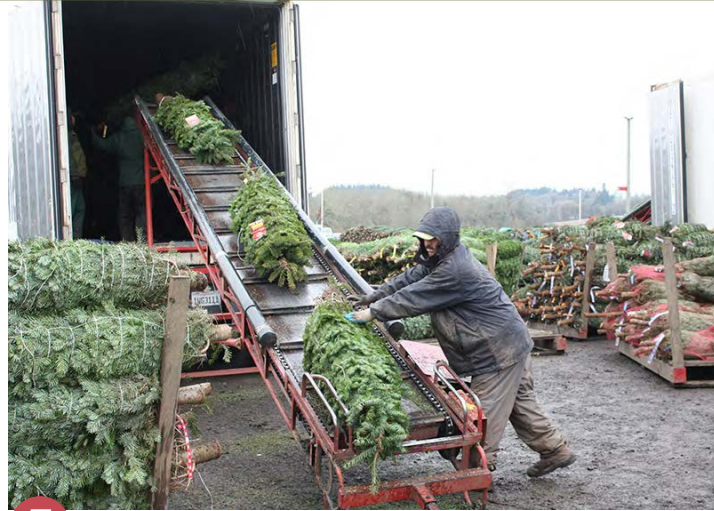
5 A conveyor belt helps transport the trees onto a truck, where they are stacked and ready to ship.
