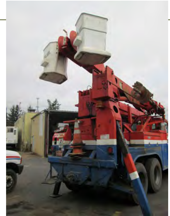
Above: The onboard aerial work platform has two buckets side by side at the end of the boom.
