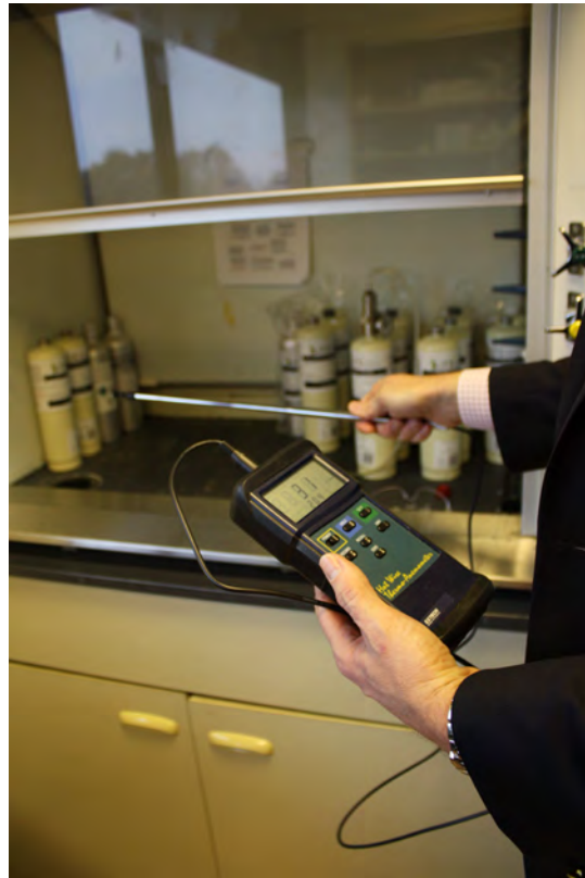
Above: Air sampling pumps are used routinely to collect air samples in different types of work settings. Right: Johnson uses a velometer to measure the air flow into a laboratory fume hood.
