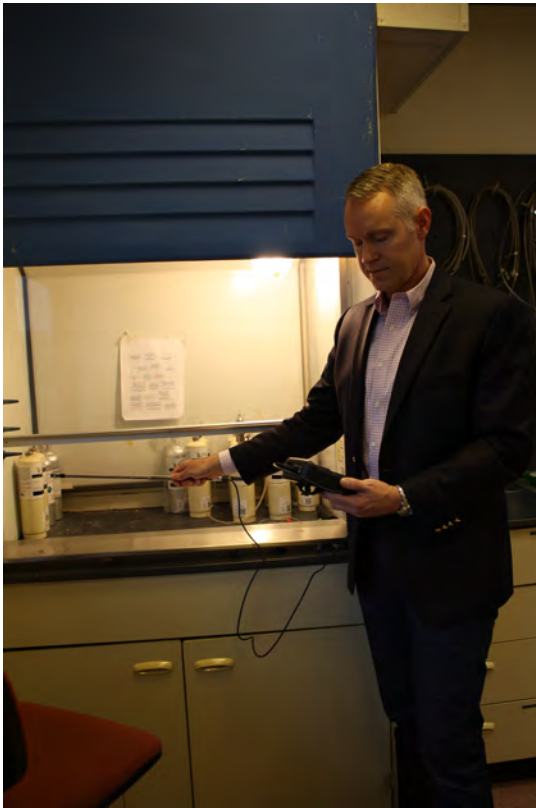
Above: Air sampling pumps are used routinely to collect air samples in different types of work settings. Right: Johnson uses a velometer to measure the air flow into a laboratory fume hood.
