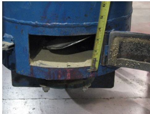
The 6-inch by 3-inch inspection hole.
