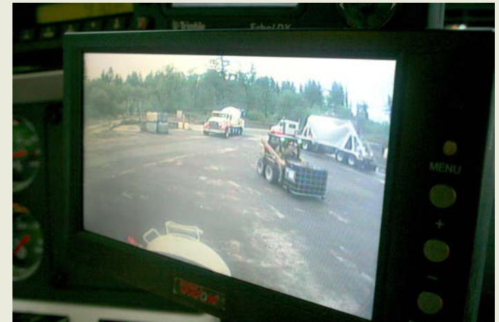
A camera installed on a Knife River ready-mix truck gives this driver a view of activity behind him.
