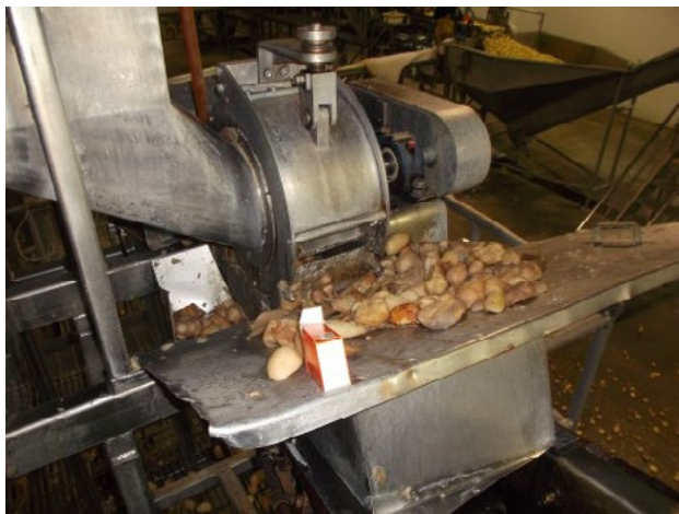
The unguarded opening to the cutting machine.
