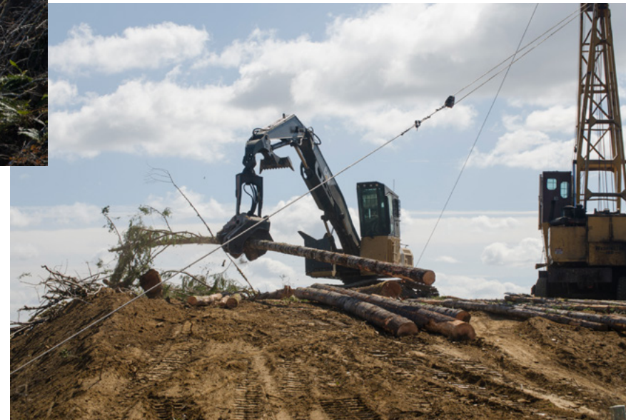
The Coos Bay Timberlands operation includes mechanized yarders, processors, and loaders that pull, strip, saw, and stack logs.
