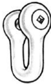
Figure 7-12 – Shackle – Flush Pin, Straight Side
