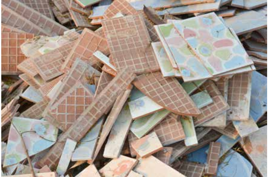
Broken asbestos floor tiles
