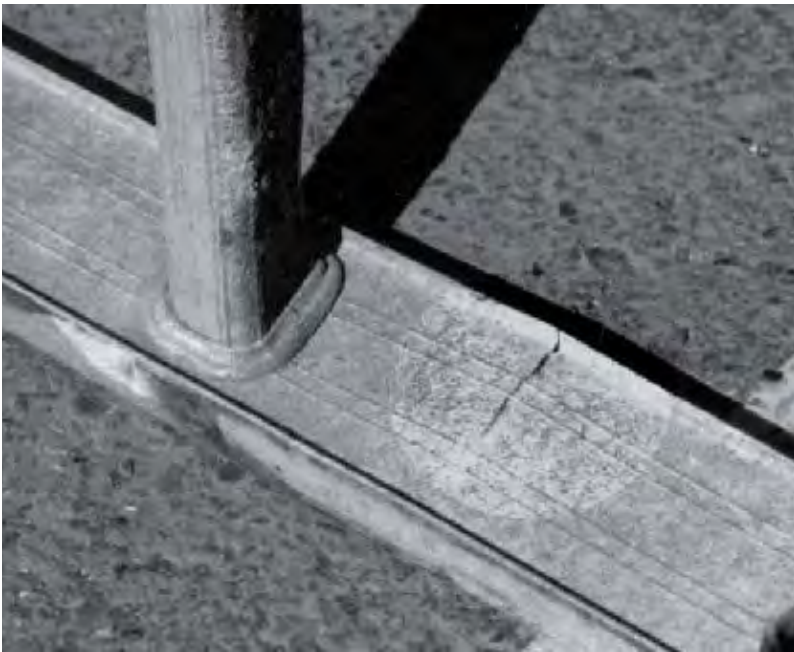
Equipment inspections are critical. Do you see the small fracture in this picture? This should not be used.
