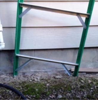
*In this photo, a standard stepladder's right rear foot unexpectedly punched through the soil's surface and into a mole's tunnel that was along a home's foundation. The employee was on the ladder's highest standing level when the ground failed, causing the employee to fall to the ground and sustain injuries. An accident investigation quickly revealed several mole holes around most of the foundation's perimeter. The injuries could have been avoided with a quick check of the ground conditions.*
