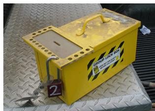
*The lockbox where the designated person placed the key to the energy-isolating devices.*
