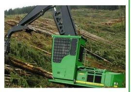
newer machines or be limited to the operating surface conditions listed above. They may also be used as an anchor for a cable yarding system where there is a clear path of travel and slopes are limited to 40 percent or less.
