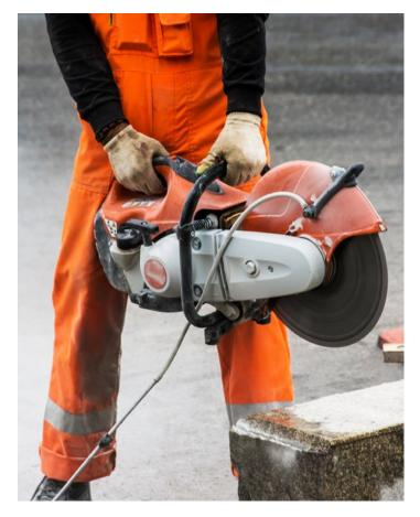
When working with handheld power saws of any blade diameter, respiratory protection with a minimum assigned protection factor (APF) of 10 is required for outdoor work more than four hours per shift and for work done indoors or in an enclosed location.
