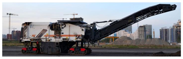
Employers whose employees operate large milling machines have two engineering control options for cuts of four inches in depth or less on any substrate and one control option for cuts of any depth on asphalt. Regardless of the option, the machine must be operated and maintained to minimize dust.
