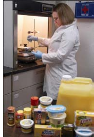
At LabCor, a Seattle analytical laboratory, analyst Eryn Knaack heats cooking oils and butter substitutes to see how much diacetyl is released. (Photo by Andrew Schneider) (December 21, 2007)
